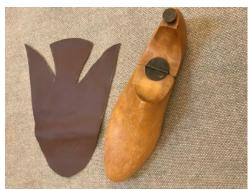
I use this one after I have measured the foot and made a pattern on the leather. This is the last around which I shape the top of the shoe.
