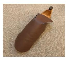
I stretch and shape the leather using these pincers, and I stitch and tack the top to a wooden or extra strong leather sole. To finish off I polish and blacken the shoes with a mixture of bee's wax and soot.
